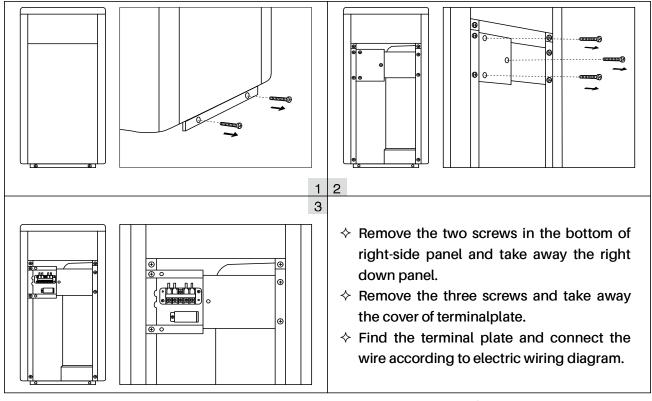
Note: For VortexPro 10~ VortexPro 13 model, please open the back panel for power connection. The operation is the same as above.
