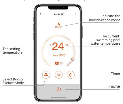
2. For heat pump with Heating&Cooling function:
