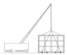
d. Do not lift the water union, otherwise, the titanium heat exchanger inside the heat pump may be damaged.
