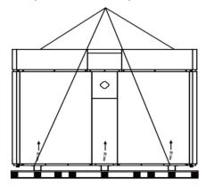
c. Transported by a crane, the sling should handle at least 1260KG
