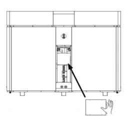
4 Align the panel with the buckle and slide up
