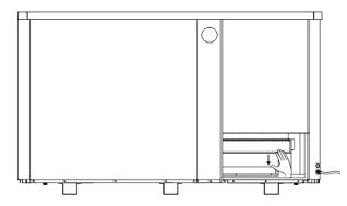
3 Fix the internal panel by two screws
